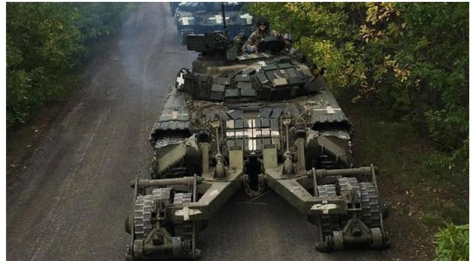
According to a post on the Ukrainian military blog NIP Tysk one of the Ukrainian columns pressing southeast towards Izyum on the M03 highway was spearheaded by a specially modified T-64A tank equipped with a minesweeper, a variant informally dubbed the BMR-64, after the BMR-2 and BMR-3 Soviet mine-rolling tanks.
