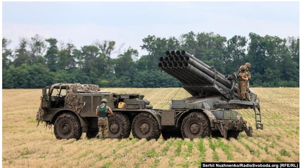
The Bureviy sits on a Tatra T815-7T3RC1 heavy, high-mobility vehicle chassis with an 8x8 configuration but fitted with a four-door armored cabin. This vehicle was specially designed for military applications and its maximum speed is 85 kilometers per hour. It is equipped with a new, digital fire-control system. It can fire all the standard Soviet-made 220-millimeter unguided rockets.
