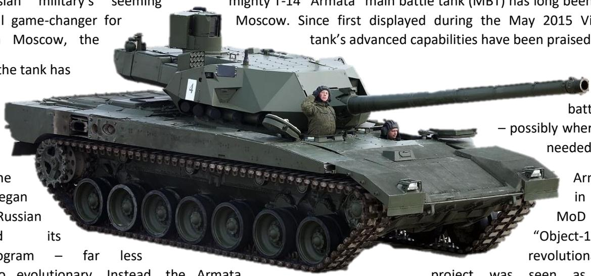
The outline of the tank, from its hull to its long and boxy turret – which resembles Western tank turret designs – was a notable departure from past Soviet designs. The T-14 also featured seven road wheels, instead of the six wheels that were commonplace on almost all previous Cold War Soviet and even modern Russian MBTs.
