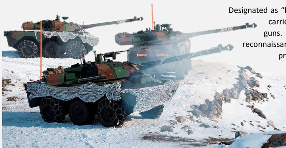
Designated as “light tanks” in French, the AMX-10 RC carries a 105mm cannon and two machine guns. It’s primarily designed for reconnaissance missions and has enough armor to protect against light infantry weapons, according to the French ministry. They have wheels rather than tracks, allowing for better mobility than heavy tanks.
