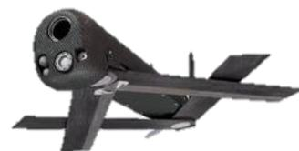
The Switchblade 300 has a range of 10 km and an endurance of just 10/15 minutes, but it has the advantage of being easily transported by a soldier in a backpack, weighting just 2.5 kg. On the other hand, the Switchblade 600 is much larger, weighting more than 22 kg, but it also offers improved performance with a range of more than 90 km and an endurance of more than 40 minutes.
