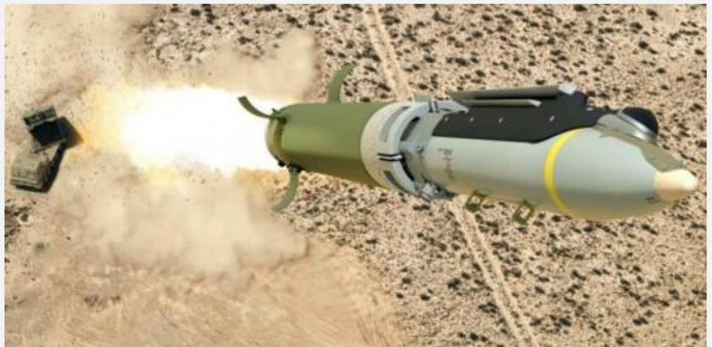
A joint project by Saab and Boeing, the GLSDB marries two affordable, combat-proven systems: the GBU-39 Small Diameter Bomb, a 113 kg precision-guided munition that is relatively cheap at around \$40,000 each, and the M26, a low-cost, formerly demilitarized rocket. The system could include a multi-purpose warhead tailored for fixed, hardened, low collateral damage, and moving targets.
